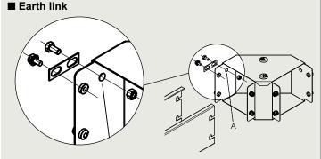
All fittings have 7 mm knockouts (A) for fixing an earth link An M5 screw and nut are needed for fixing the earth link
