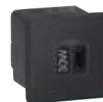
USB Type-C port with 30W power delivery
