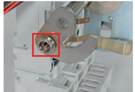
Place the centering ring on the left side of the rotation axis and screw the guiding plate of the circuit breaker rack to the left of the base.
