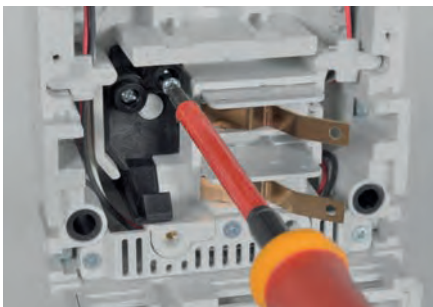
Mount the draw-out system starting with the right side of the base (do the mounting with the base laid flat). Position the rotation shaft and the guiding plate of the circuit-breaker rack on the right-hand side of the base, then fix the drive stud with its centring ring, and verify that the shaft rotates correctly in both directions. Fix the draw-out system to the guiding plate of the circuit-breaker rack already installed by screwing in 4 screws (tightening torque 2 Nm), and verify that the rotation axis is correctly positioned inside it.
