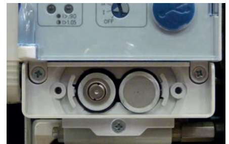
The battery compartment, located underneath the electronic protection unit, is accessible from the front panel
