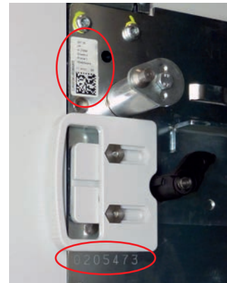
On the right side of the DMX 3 , the end of the serial number is engraved on the metal structure and is shown in full, with the date of manufacture on a sticker.
