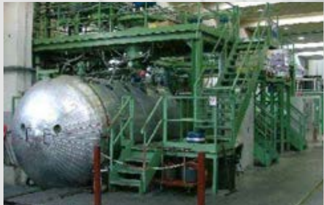
The pouring system under high vacuum
